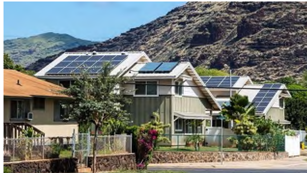
Figure 1. Distributed solar—solar panels installed on customer rooftops. 4
