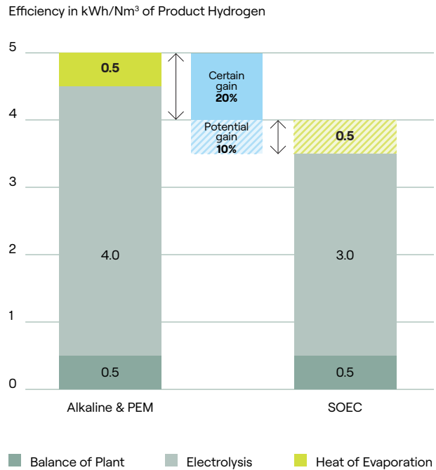
FIGURE 2: SOEC'S ADVANTAGE OVER ALKALINE AND PEM TECHNOLOGIES
