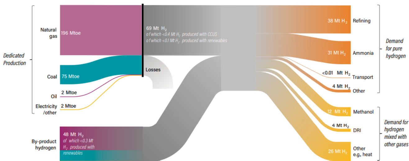
Figure 1. The global hydrogen value chain (2018) shows the dominant use of hydrogen is oil refining and ammonia production. Transportation is an emerging opportunity. Source: (John Feldmann, 2023), (IEA, 2019)
